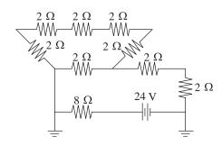
What is the current through the 8  $\Omega$  resistor in the circuit shown above?
