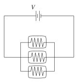
Three identical light bulbs are connected to a source of emf, as shown in the diagram above. What will happen if the middle bulb burns out?
