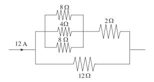
What is the voltage drop across the 12  $\Omega$  resistor in the portion of the circuit shown above?
