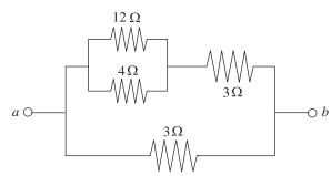
Determine the equivalent resistance between points a and b.
